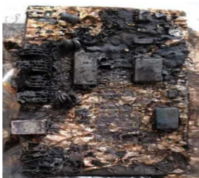
Fig. 1. Waste printed circuit board (PCB) after gasification in a steam atmosphere [12]
